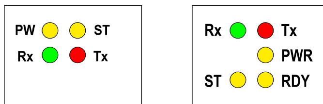
Fig. 5 – LEDs on modules with the CAN interface
